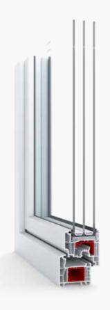
In a configuration with the new half-recessed sash, with the option of glazing with glazing units up to 48 mm wide, it is possible to create even warmer window constructions in the IDEAL 4000 system (up to U<sub>w</sub>=0.85 W/m²K).
